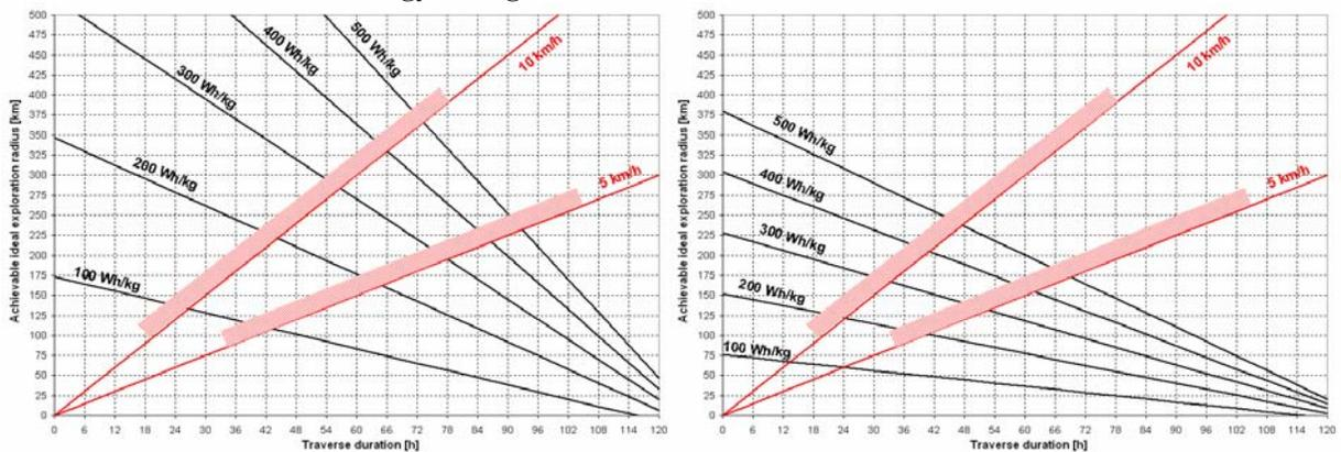
**Figure 8: Ideal exploration radius from a planetary surface base as a function of energy storage density for a pair of pressurized rovers with one energy storage trailer each; lunar surface environment (left) and Mars surface environment (right).**
