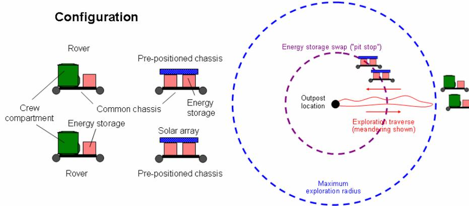
**Figure 5: Pressurized mobility concept based on the use of two independent pressurized vehicles and two pre-positioned chasses with power systems and consumables (one or more pre-positioned chasses per rover)**
