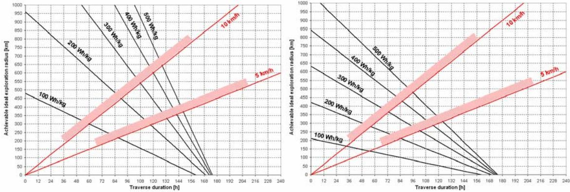
**Figure 11: Ideal exploration radius from a planetary surface base as a function of energy storage density for a pair of pressurized rovers with two optimally pre-positioned power and consumables stations each; lunar surface environment (left) and Mars surface environment (right).**
