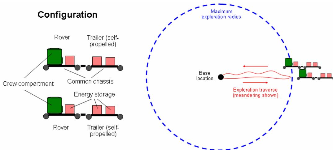
**Figure 4: Pressurized mobility concept based on the use of two independent pressurized vehicles as well as trailers with additional energy storage for extended range operations (one or more trailers per rover)**
