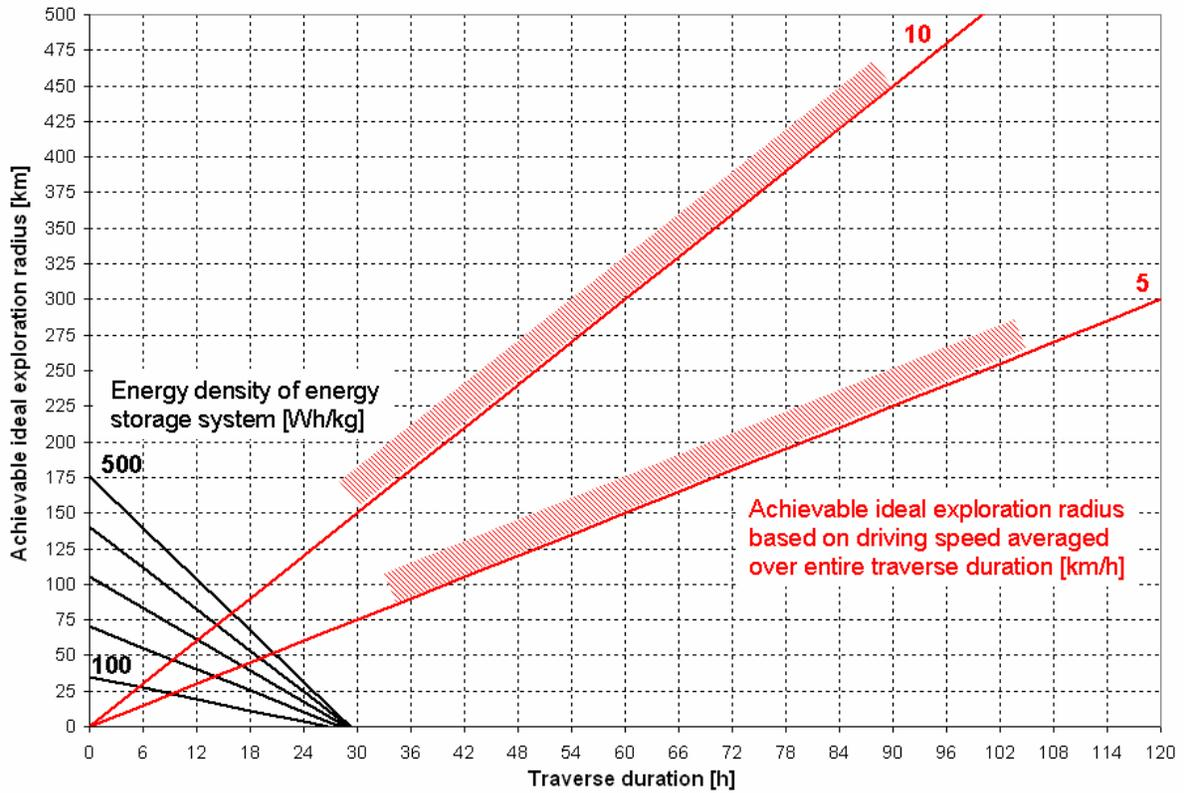
Figure 15: Mars surface ideal exploration radius, 2 pressurized rovers
