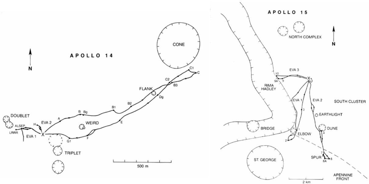
**Figure 1: Comparison of Apollo 14 surface traverses on foot (left side) with Apollo 15 surface traverses using the Apollo LRV (right side)<sup>3</sup>; note the different levels of scale (500 m vs. 2 km)**
