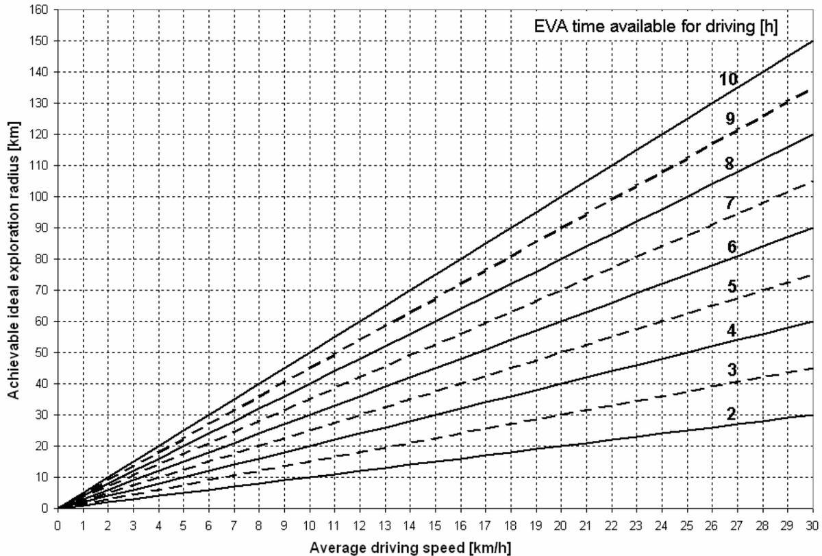
**Figure 6: Ideal exploration radius accessible from a Moon or Mars surface base using two independent unpressurized vehicles as a function of average driving speed and the EVA time available for driving**
