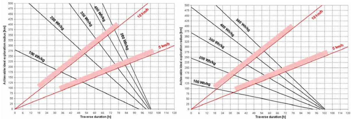
**Figure 10: Ideal exploration radius from a planetary surface base as a function of energy storage density for a pair of pressurized rovers with one optimally pre-positioned power and consumables station each; lunar surface environment (left) and Mars surface environment (right).**
