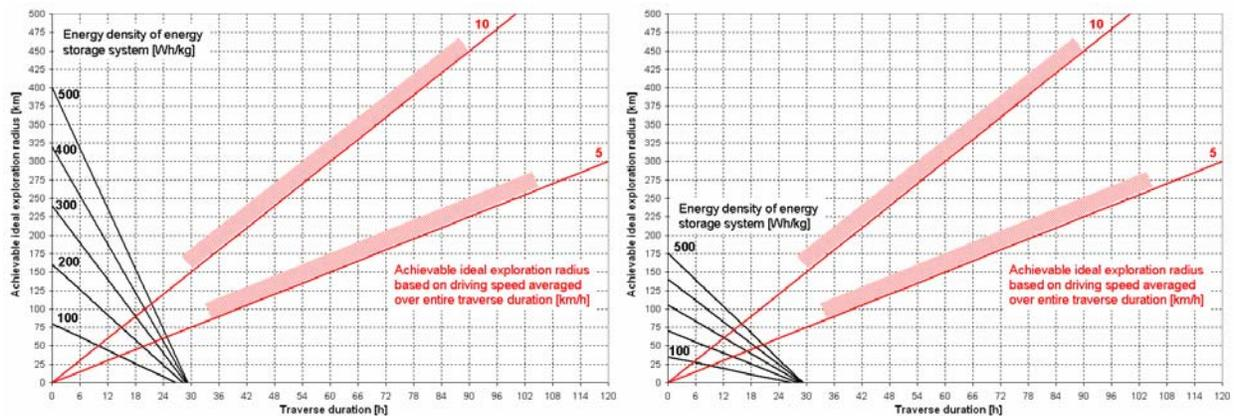
**Figure 7: Ideal exploration radius from a planetary surface base as a function of energy storage density for a pair of pressurized rovers; lunar surface environment (left) and Mars surface environment (right). Also shown are the limits to exploration range based on driving speed averaged over the entire traverse duration.**
