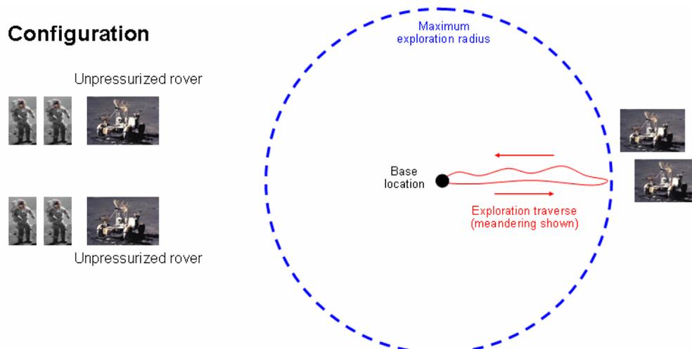
**Figure 2: Unpressurized mobility concept based on the use of two independent unpressurized vehicles capable of carrying the entire crew back to base in the event of an emergency / contingency (images courtesy NASA)**
