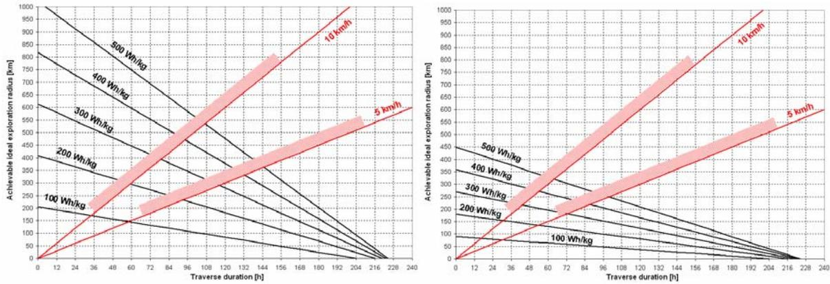
**Figure 9: Ideal exploration radius from a planetary surface base as a function of energy storage density for a pair of pressurized rovers with two energy storage trailers each; lunar surface environment (left) and Mars surface environment (right).**
