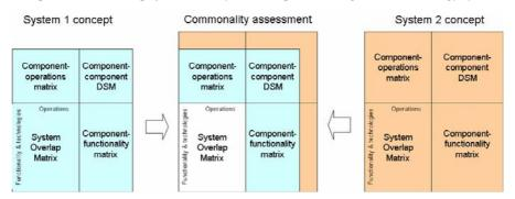
Figure 4: Coupling of SOM to component-component DSM via component-operations / functionality matrices for identification of opportunities for architectural and design commonality
