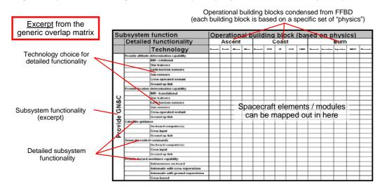
Figure 2: Excerpt from the System Overlap Matrix template for a spacecraft
